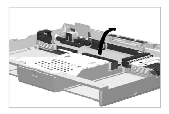
Figure 5-59. Removing the System Board
